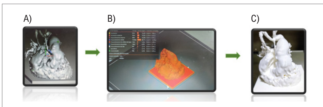
Figure 3 – Construction of 3D models: a) cleaning and smoothing carried out using the software; b) estimated model for production by the printer; c) produced model (original figures).
